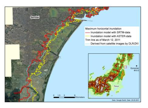
Figure 5: Comparison of modelled inundation based on ASTER GDEM and SRTM for a test scenario (figure produced by Lasse Scheele).
