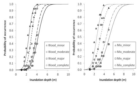
Figure 12: Fragility functions developed from the Tohoku tsunami for Miyagi prefecture developed by Suppasri et al. (2012b).
