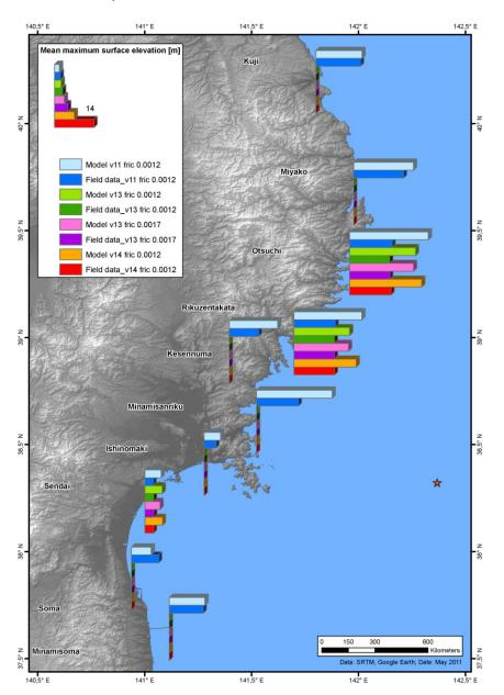
Figure 7: Model runs for scenario D (dispersive) based on different values for bottom friction. The model results are compared to the field observations for each bar (figure produced by Lasse Scheele).
