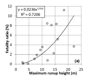
Figure 16: Relationship between maximum run-up height and fatality ratio based on data from Miyagi prefecture (Suppasri et al., 2012a).
