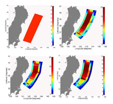
Figure 1: Slip distribution for the four different earthquake source scenarios A-D. Upper left, scenario A, Mw 8.89. Upper right, scenario B, Mw 8.85. Lower left, scenario C, Mw 8.95. Lower right, scenario D, Mw 8.87 (Løvholt et al. 2012).
