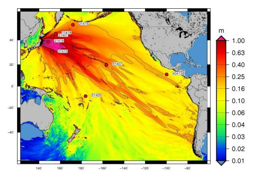
Figure 3: Maximum surface elevation for scenario D and DART locations for the entire Pacific Ocean, dispersive solution. Contour lines are drawn for every 20 cm (Løvholt et al. 2012).
