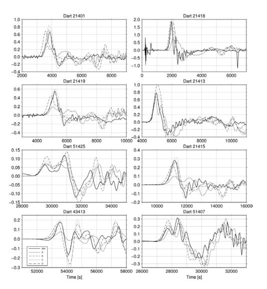
Figure 4: Source sensitivity for a range of DART locations exemplified for scenarios A-D, dispersive solution (Løvholt et al. 2012).
