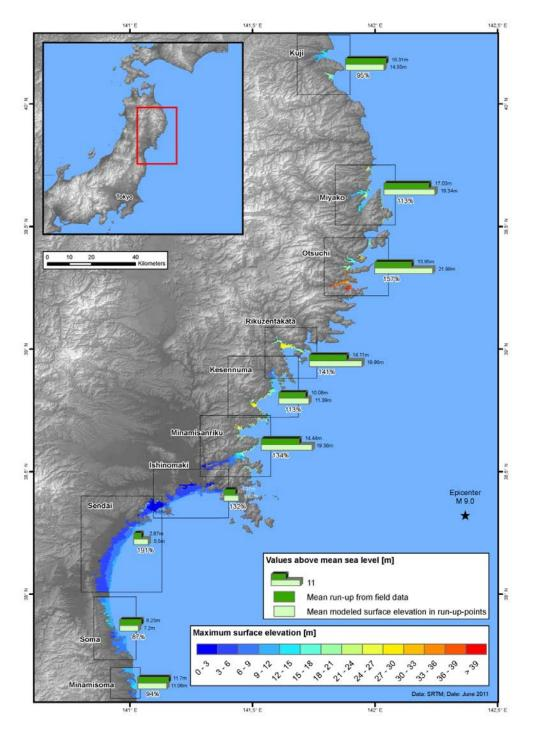
Figure 8: Comparison of the modeled maximum surface elevation of scenario D (dispersive) with field measurements published by the Coastal Engineering Committee of the Japan Society of Civil Engineers (2011). Mean values summarizing point measurements in each study area and the corresponding mean values of the modeled surface elevation in these points are shown (Løvholt et al. 2012).
