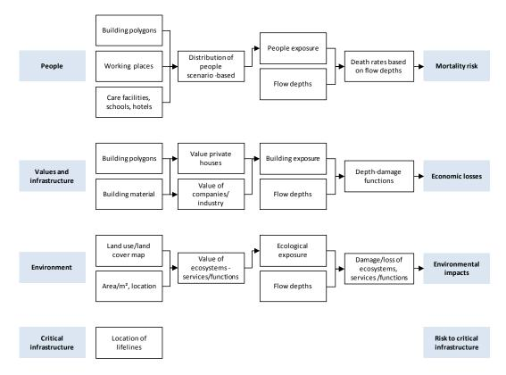
Figure 18: Sketch on the overall approach for tsunami risk assessment.
