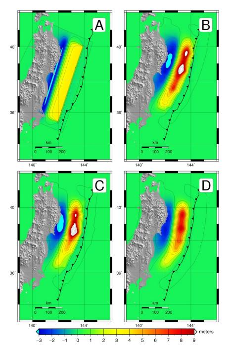
Figure 2: Initial surface elevations for the four different earthquake source scenarios A-D (Løvholt et al. 2012).
