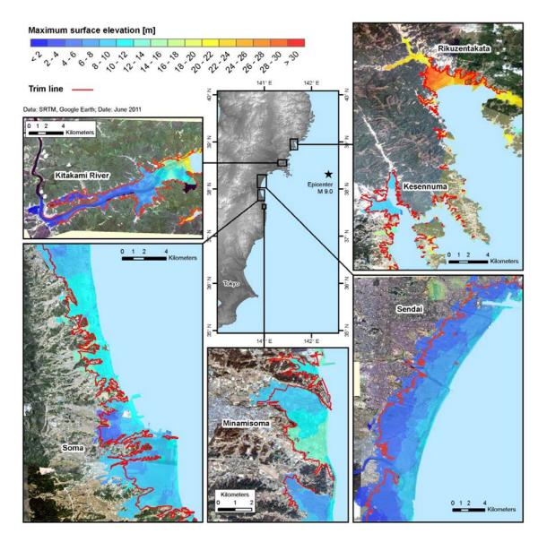
Figure 9: Comparison of the maximum modelled inundation extent (scenario D dispersive) with trim lines derived from pre-/post-tsunami satellite images by the Tsunami Damage Mapping Team, Association of Japanese Geographers (2011). Results are shown for the Kitakami River close to Minamisanriku, Soma, Kesennuma, Minamisoma, and Sendai (Løvholt et al. 2012).
