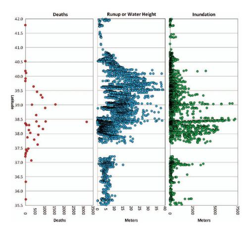
Figure 13: Latitude-based graphs of total deaths for selected principalities and prefectures, run-up or maximum water height, and maximum inundation distance from the 2011 Tohoku tsunami (Source: Dunbar et al. 2011, after IOC 2011 – deaths; Mori et al. 2011 – run-up or water height and inundation distance).
