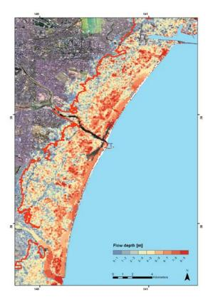
Figure 15: Total water depth in Sendai. Map generated by a subtraction of the modelled surface elevation and the SRTM elevation model (figure produced by Lasse Scheele).
