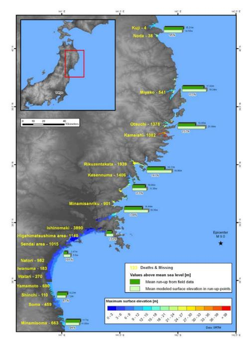
Figure 10: Number of fatalities by community (based on EERI 2011) combined with mean measured and modelled run up (scenario D dispersive) (modified from Løvholt et al. 2012).
