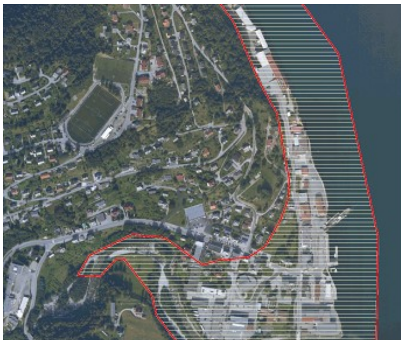
Fig. 3.14: Example of hazard map for tsunamis from a potential rockslide at Åkerneset impacting Stranda, Sunnylvsfjorden. (Hazard zone up to 10 m.a.s.l., produced by the Åknes/Tafford project) (Source: Harbitz et al., Rockslide tsunamis in complex fjords: From an unstable rock slope at Åkerneset to tsunami risk in western Norway. 2014)
