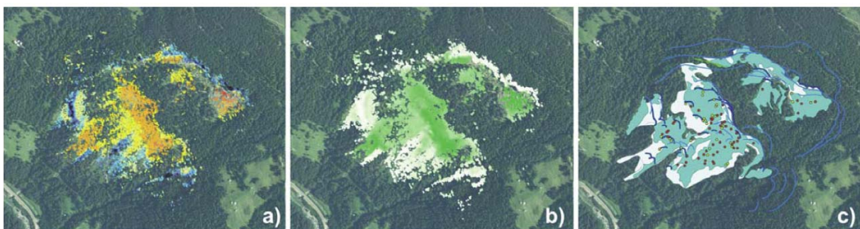
Figure 4.11-10. Steps toward the identification of rockslide sub-areas: a) reclassification of CD maps; b) smoothing of CD maps by neighbourhood statistical techniques; c) comparison to geological and geomorphological field evidence (e.g. slope material, style of activity).
