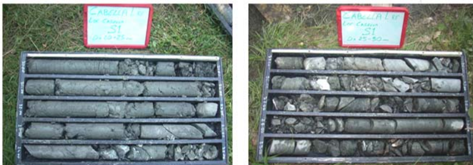
Figure 4.6-2. Stratigraphy sketch and coring of Casella S1/2009 borehole.
