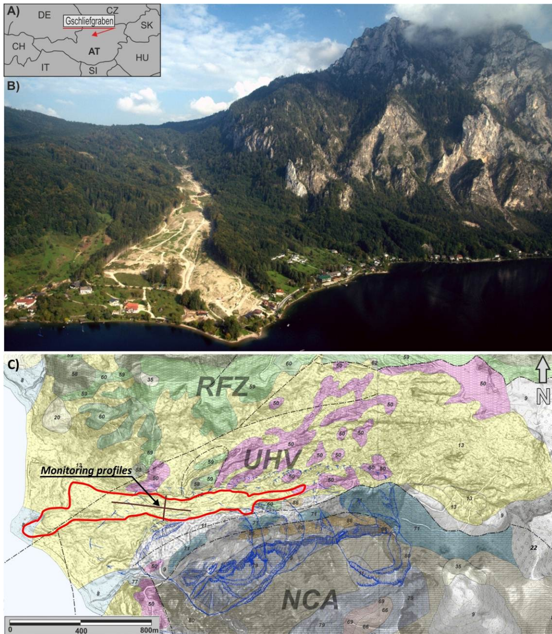
Figure 4.7-1. General setting of the Gschlifgraben site: (A) Position within Austria, (B) Airborne photo of the Gschlifgraben valley and Mt. Traunstein from the west (Photo: R. Supper, 2009), and (C) Geological map of the area of Gschlifgraben. The blue contours indicate the Deep-seated gravitational deformations. Legend: Quaternary deposits: 8 - Alluvial Fan, 9 - Slope Scree, 11 - Block Fields, 13 - Landslide Deposits, 20 - Glacilacustrine deposits, 22 - Slope Breccia, 35 - Moraine deposit; UHV: 50 - Buntmergel Fm., 52 - Greisten Fm.; RFZ: 53 - Altliengbach Fm., 57 - Perneck Fm., 58 - Zementmergel Fm., 59 - Seiesenburg Fm., 60 - Rieselsberg Fm., 62 - Gaultflysch Fm.; NCA: 66 - Schrambach Fm., 69 - Ruhpolding Fm., 71 - Calcarenite Fm., 75 - Koessen Fm., 76 - Koessen Fm., 77 - Koessen Fm., 79 - Plattenkalk Fm., 80 - Hauptdolomit Fm.; the major tectonic faults are as dot-and-dashed lines (modified after Egger et al. 1996, Egger et al. 2007 and Moser et al. 2009).
