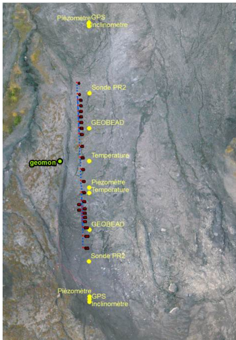
Figure 4.13-6. Layout of the geoelectrical monitoring profile: red=current electrodes, blue=potential electrodes, yellow=other sensors (north orientation is towards the top; Source: Google Earth).
