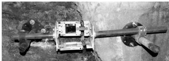
**Figure 5: The TM71 crack gauge installed underground to bridge a joint. It is equipped with two planar moiré indicators in two perpendicular planes, horizontal xy, and vertical xz, that define 3D displacement between the two joint faces in the wall. The TM71 crack gauge is a product of GESTRA, Sedloňov, Czech Republic.**
