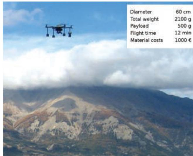
**Figure 9.** Small UAV developed by the Universität Stuttgart, used in the Super-Sauze landslide to acquire aerial images with small compact cameras (Walter et al., 2009).
