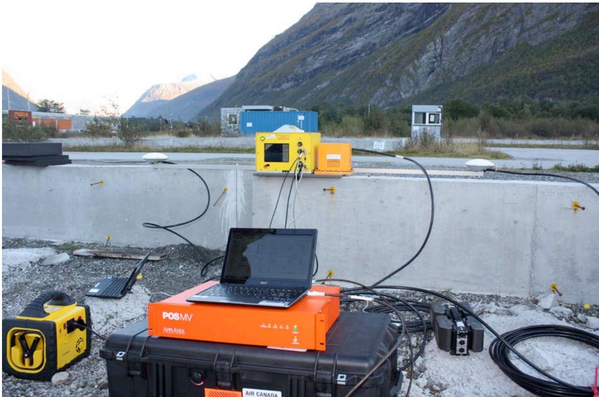
**Figure 119: Onshore calibration of the coupled TLS Optech ILRIS-3D-ER with the IMU/GNSS Applanix POS MV.**
