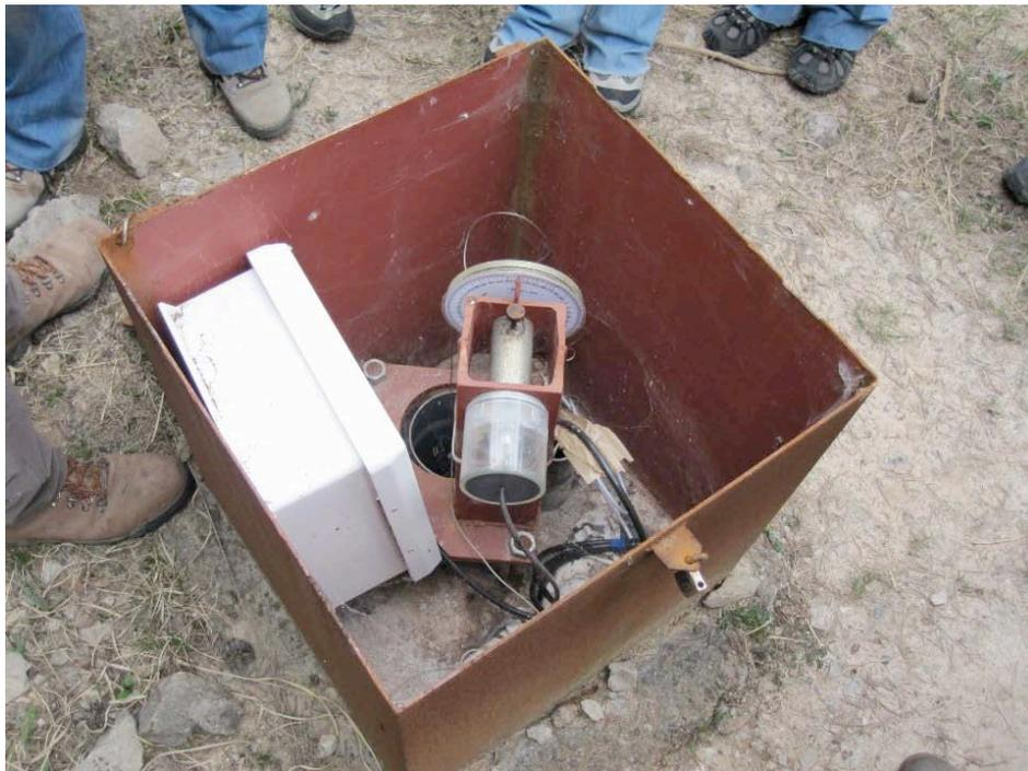
Figure 2: View of the upper part of the wire extensometer. In the centre, the pulley, the dial and the potentiometer.
