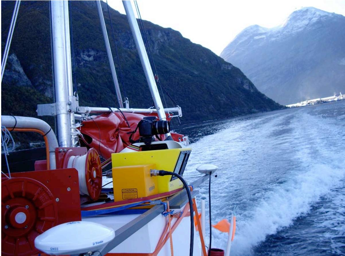
**Figure 120: Offshore acquisition with the OLS system setup on a boat, in the Norwegian fjord.**
