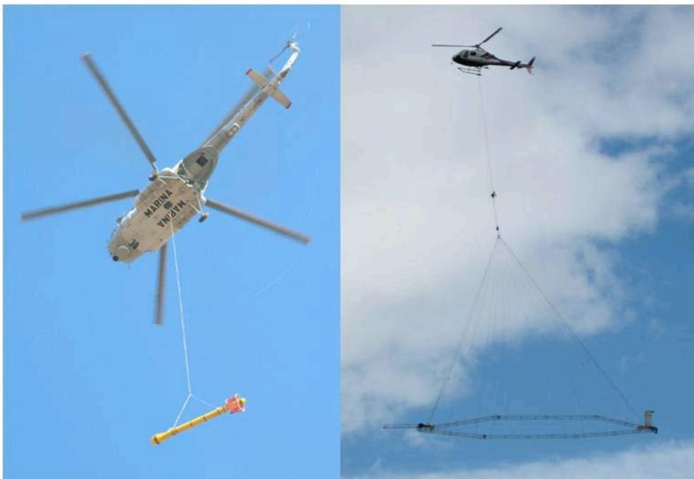
**Figure 15.** Left: helicopter borne electromagnetic (HEM) system; right: helicopter borne skytem system (photos: R. Supper, 2009).
