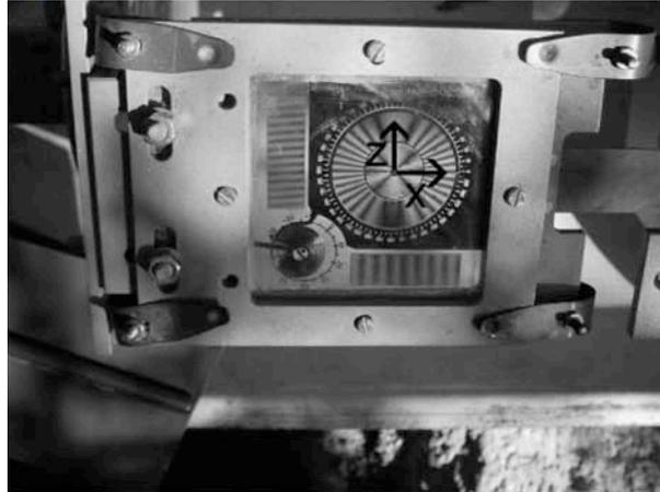
**Figure 6: A view of one of the TM71 indicators, in detail. The indicator shows several moiré patterns and a spiral thermometer. Displacement vectors in the vertical plane XZ are defined by the actual positions and densities of the moiré fringe patterns. The thermometer serves for calculations needed to compensate for temperature variation effects.**
