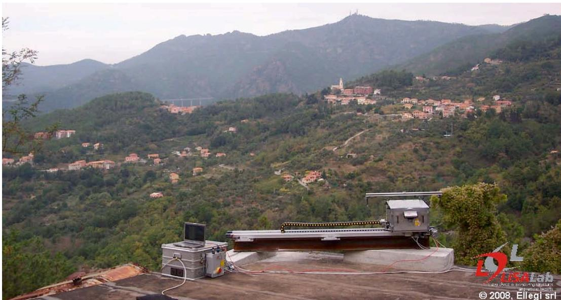
**Figure 84. Close-up view of the GB-InSAR system installed in front of the monitored area.**
