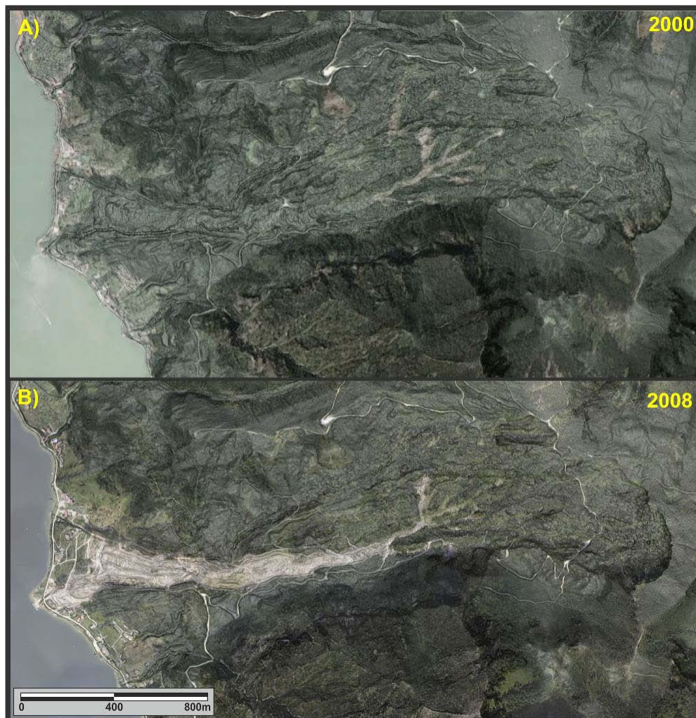
Fig. 3: The activity of the earthflow complex between 2000 and 2008 was assessed based on the identification of bare surfaces on set of orthophotos. The orthophotos are superimposed on the ALS pseudo-hillshade.
