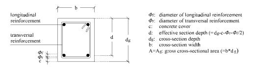
Figure 2.4 Cross section of the column
