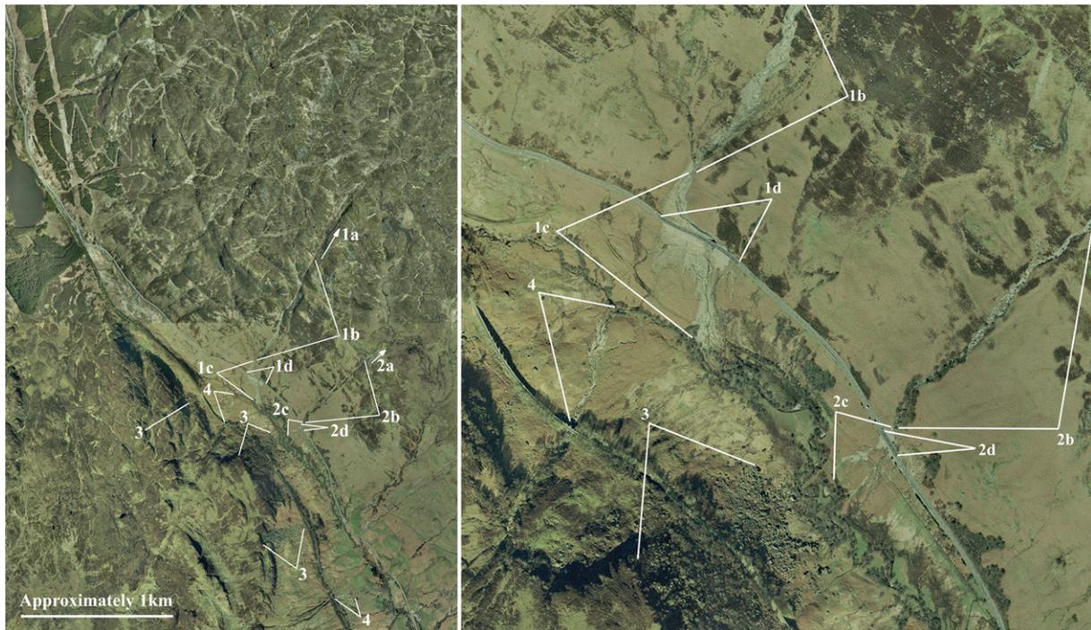
**Figure 4.5.21** Aerial photographs (north to the top) showing the Glen Ogle debris flows of August 2004 showing key features (Licensed to Transport Scotland for PGA, through Next Perspectives<sup>TM</sup>): Left; 4km by 3km (12 tiles), National Grid Reference (NGR) of SW corner NN 560 250 or 2560 7250; Right; 1km by 1km (single tile), NGR of SW corner NN 570 260 or 2570 7260.
