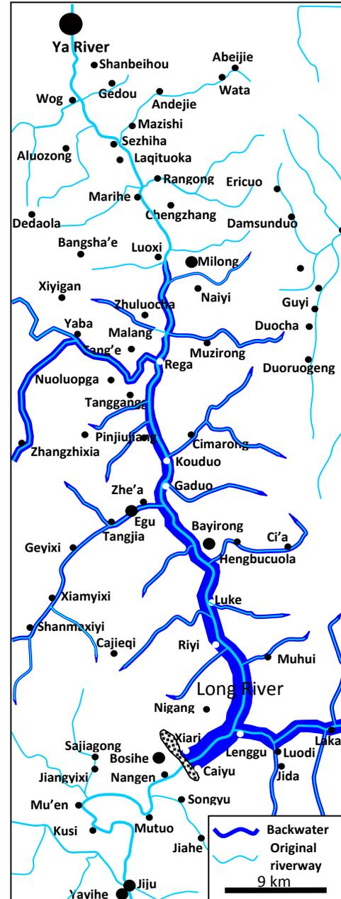
Figure.6 Tanggudong landslide dam and its backwater scope
