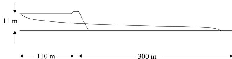
Fig. 3.4.1. Central section of the failure at Gypsum Tailings impoundment
