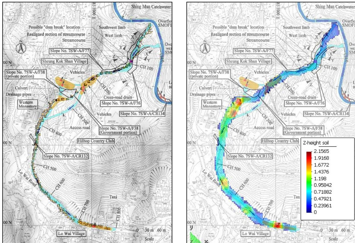
Fig. 3.3.7. Lo Wai debris flow. Computation with channeling barriers: Observation vs. Computed results
