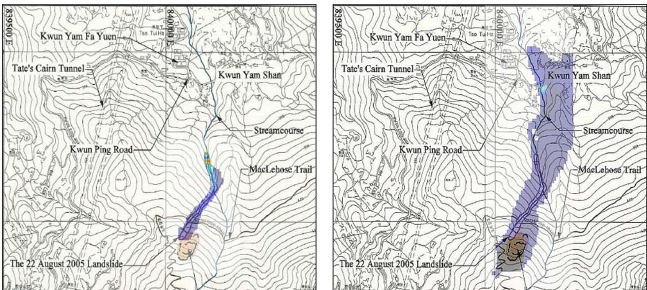
Fig. 3.2.3. Model predictions for Tate's Cairn: comparison between the results obtained with a cohesive fluid model (Bingham) for the two initial masses (i) left: 1200 m<sup>3</sup> (ii) right 10000 m<sup>3</sup>
