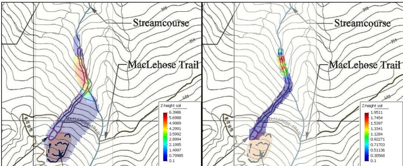
Fig. 3.2.2. Model predictions for Tate's Cairn: comparison between the results obtained with a frictional fluid (Voellmy) for the two initial masses (i) left: 1200 m<sup>3</sup> (ii) right 10000 m<sup>3</sup>
