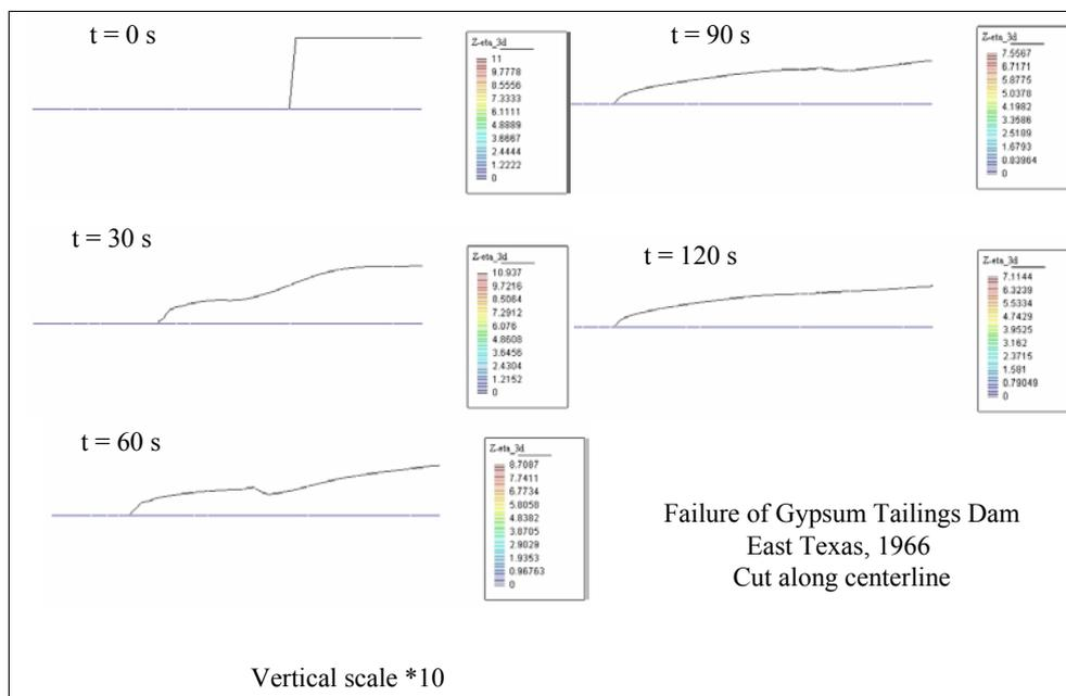
Fig. 3.4.4. Gypsum tailings dam failure: profiles along central section
