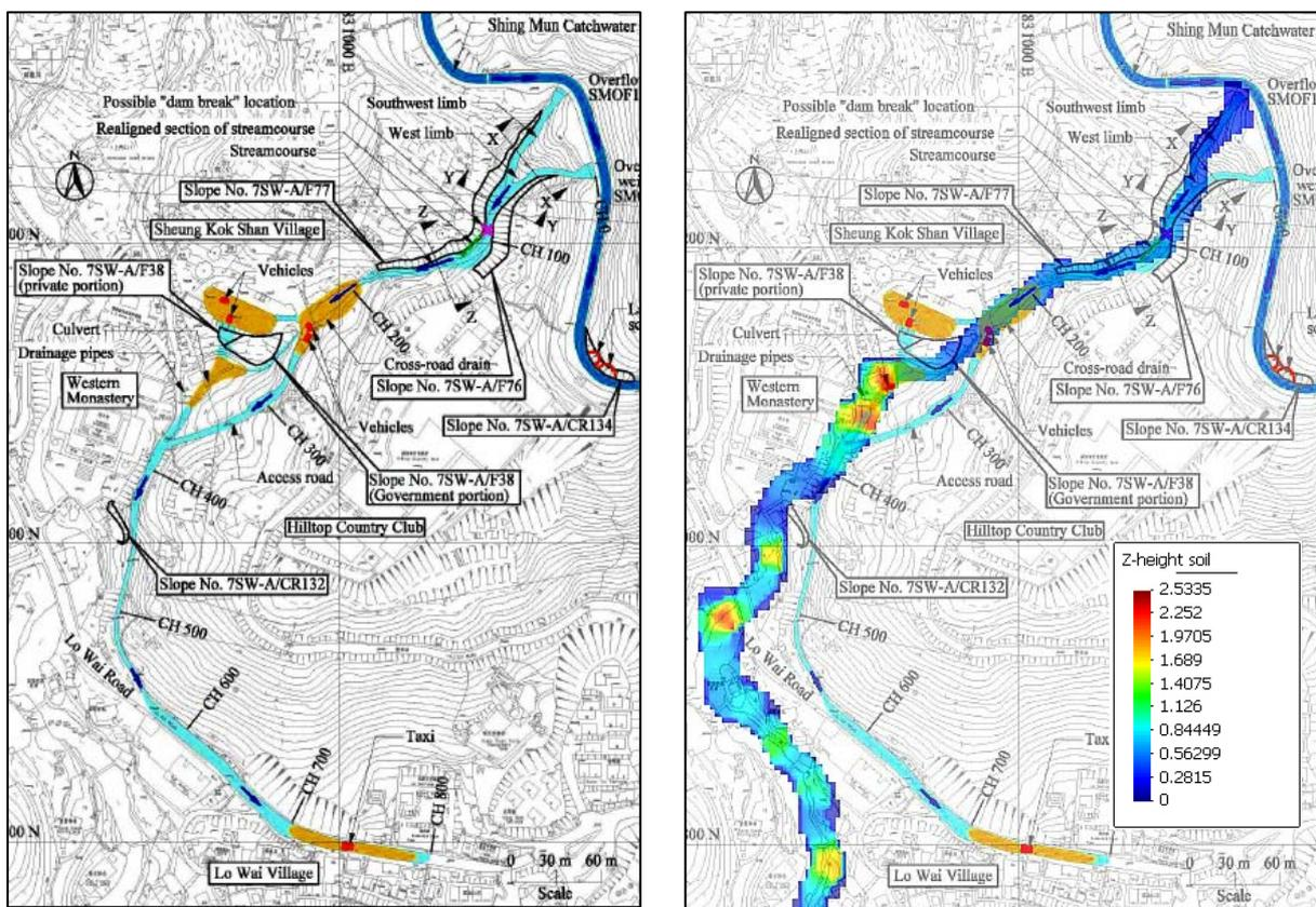
Fig. 3.3.5. Lo Wai debris flow. Computation without channeling barriers: Observation vs. Computed results
