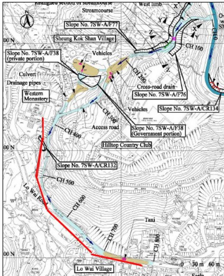
Fig. 3.3.6. Lo Wai debris flow. Computation Location of the computational channelling barriers
