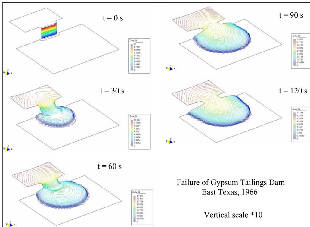
Fig. 3.4.3. Run out of Gypsum tailings dam failure
