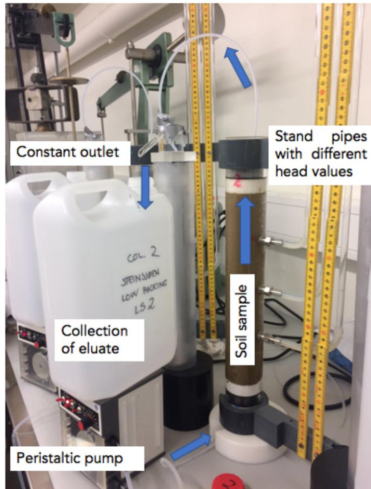
**Figure 15.** Setup for the lightly packed shooting range soil, L/S ratio 2. Deionized water was pumped into the column using a peristaltic pump, and eluates were collected in plastic containers. The calculation of the hydraulic conductivity from the stand pipes is described in Section 4.6.1 *Calculation of hydraulic conductivity from the extended up-flow percolation columns.*
