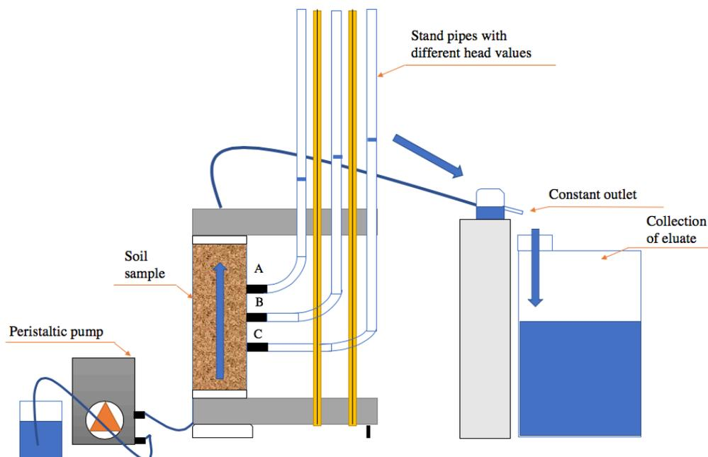
**Figure 13.** Experimental setup for the extended up-flow percolation columns. The eluent was pumped from the bottom towards the top of the soil column using a peristaltic pump (arrow in the column indicates flow direction). Eluate was collected for chemical analysis. The stand pipes allow the hydraulic conductivity to be calculated.
