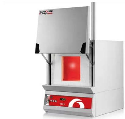
Fig.1 Ashing Furnace used for experiments.
