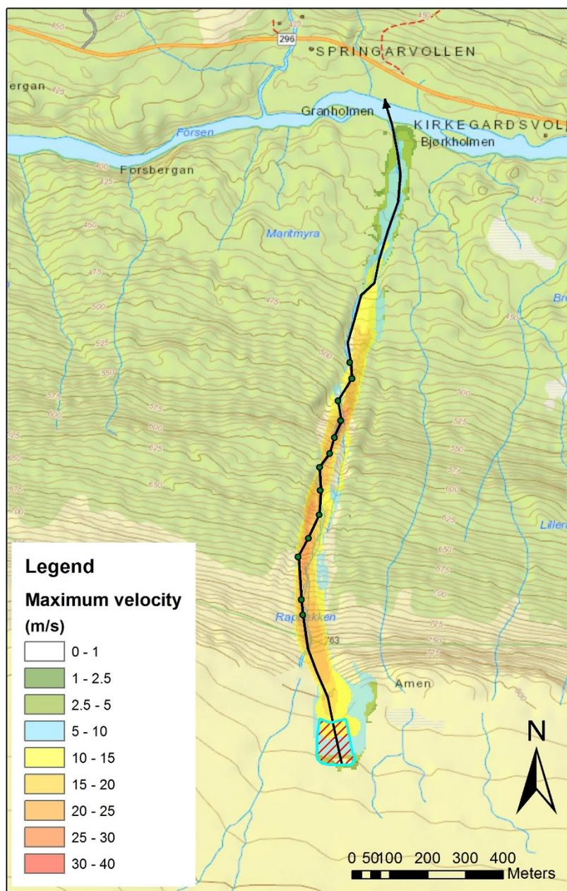
Figure 2. Back-calculation of the slushflow event in Skarmodalen on 2010-05-16 using RAMMS with  $\mu = 0.05$  and  $\xi = 2000 \text{ m s}^{-2}$ . The chosen release height  $d = 1.5 \text{ m}$  leads to a total release volume of approx.  $15,300 \text{ m}^3$ .
