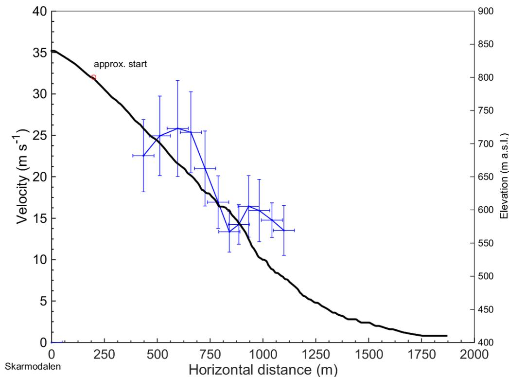
Figure 1. Measured front velocity of the slushflow in Skarmodalen, 2010-05-16. From Deliverable D3.1 in the 2014 report on WP3.
