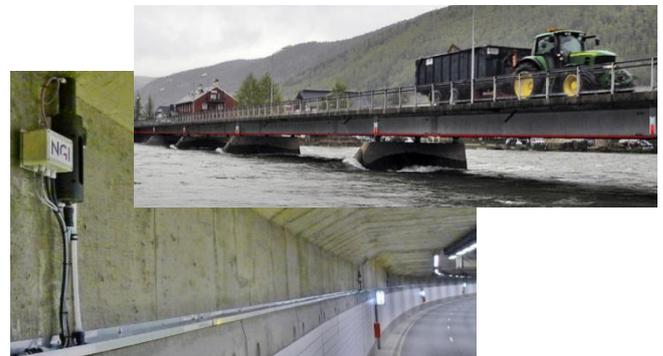
**NGI's automatic Hose level system mounted in Bjørvika (E18 Oslo) submerged tunnel for settlement monitoring (above left)**
